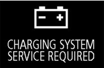
If there is a fault with the charging system, the warning display is displayed on the information screen in the multi-information display. The warning lamp in the instrument cluster also illuminates.
