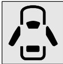
This lamp illuminates when a door or the tailgate is either open or not completely closed. If the vehicle speed reaches approximately 8 km/h with a
