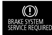
When the operation mode is put in ON, if the brake fluid is low, this warning is displayed.
