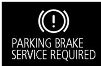
If there is a malfunction in the system, the Electric parking brake warning lamp (yellow) will come on. In addition, the warning display appears on the information screen in the multi-information display.
