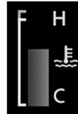
This indicates the engine coolant temperature.
