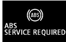
If there is a malfunction in the system, the ABS warning lamp will come on and the warning display will appear on the information screen in the multi-information display. Under normal conditions, the ABS warning lamp only comes on when the ignition switch is turned to the “ON” position or the operation mode is put in ON and goes off a few seconds later.
