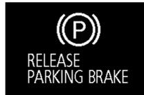
This warning is displayed if you drive with the parking brake still applied. The warning lamp in the instrument cluster also illuminates when the parking brake is applied.
