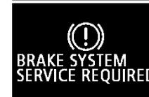
The ABS and brake force distribution function may not work, so hard braking could make the vehicle unstable. Avoid hard braking and high-speed driving. Stop the vehicle in a safe place immediately and contact an authorised MITSUBISHI MOTORS dealer.
