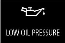
If the engine oil pressure drops while the engine is running, the warning display is displayed on the information screen in the multi-information display.
