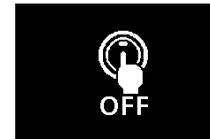
When the operation mode is in any mode other than OFF, if you try to lock the doors and the tailgate by pressing the driver’s or front passenger’s door lock/unlock switch, or the tailgate lock/unlock switch, warning display will appear and the outer buzzer will sound and you cannot lock the doors.
