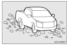
Set the 4WD selector to "4H" or "4L" position (Easy Select 4WD), "4HLc" or "4LLc" position (Super Select 4WD II) and drive at a low speed. Depending on the road condition, set the rear differential lock (if so equipped) to ON if the vehicle is likely to get stuck. This may help you drive smoothly.
