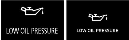
If the engine oil pressure drops while the engine is running, the warning display is displayed on the information screen in the instrument cluster.
