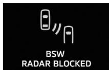
When the warning display appears, the sensor cannot detect a vehicle travelling side by side or an approaching vehicle, because foreign objects, such as dirt, snow or ice, adhere to the bumper surface around the sensor. Remove a dirt, freezing or foreign material on the bumper surface around the sensor. When the warning display does not disappear after having cleaned the sensor, contact an authorised MITSUBISHI MOTORS dealer.
