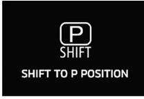
SHIFT TO P POSITION                          | <ul style="list-style-type: none"> <li>The engine is stopped while the selector lever is in a position other than the “P” (PARK) position.</li> </ul> | <ul style="list-style-type: none"> <li>Place the selector lever in the “P” (PARK) position to put the operation mode in OFF.</li> </ul>                                                        |
