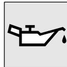
This lamp illuminates when the operation mode is put in ON, and goes off after the engine has started. If it illuminates while the engine is running, the oil pressure is too low.
