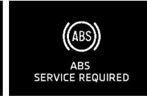
If there is a malfunction in the system, the ABS warning lamp will come on and the warning display will appear on the information screen in the instrument cluster.
