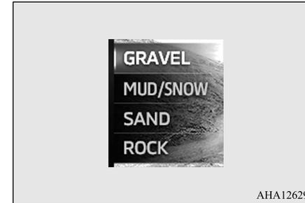
The selected control mode is displayed on the Off Road mode indicator display.
