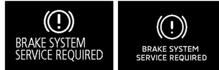
When the operation mode is put in ON, if the brake fluid is low, this warning is displayed. The warning lamp in the instrument cluster also illuminates.
