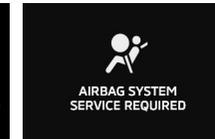
There is a supplemental restraint system (“SRS”) warning lamp on the instrument panel. The system checks itself every time the operation mode is put in ON. The SRS warning lamp will come on for several seconds and then go out. This is normal and means the system is working properly.
