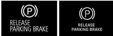
This warning is displayed if you drive with the parking brake still applied. The warning lamp in the instrument cluster also illuminates when the parking brake is applied.
