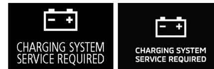
If there is a fault with the charging system, the warning display is displayed on the information screen in the instrument cluster. The warning lamp in the instrument cluster also illuminates.
