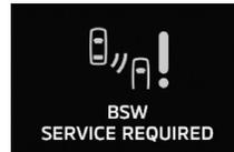
When the warning display appears, the BSW does not operate normally because there are some malfunctions in the system or the sensor. Have the vehicle inspected at an authorised MITSUBISHI MOTORS dealer as soon as possible.
