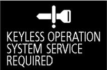
KEYLESS OPERATION SYSTEM SERVICE REQUIRED    |
