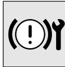
This warning lamp will illuminate when there is a fault in the electric parking brake system.
