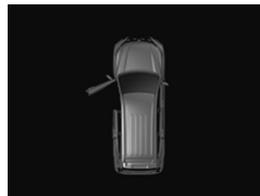
If any door or the tailgate is not completely closed, this displays the open door or tailgate. When the operation mode is ON, if the vehicle speed exceeds approximately 8 km/h while a door or tailgate is ajar, a buzzer sounds 4 times. This notifies the driver that a door is ajar.
