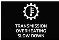
TRANSMISSION OVERHEATING SLOW DOWN         | <ul style="list-style-type: none"> <li>The A/T fluid temperature is too high.</li> </ul>                                                              | Refer to “When a malfunction occurs in the A/T” on page 6-33.                                                                                                                                  |
