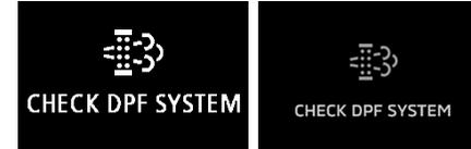
If an abnormal condition occurs in the DPF system, the DPF warning display and check engine warning lamp illuminate. Immediately have the system inspected by an authorised MITSUBISHI MOTORS dealer.
