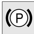
This lamp illuminates when the parking brake is applied while the operation mode is in ON.
