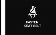
If the operation mode is put in ON while a seat belt is not fastened, the warning lamp comes on and the tone sounds for approximately 6 seconds to remind the driver and/or the front passenger to fasten the seat belt.
