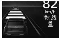
If the vehicle in front stops, the ACC reacts to it by stopping your vehicle. Depress the brake pedal as soon as your vehicle comes to a stop.
