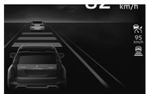
The ACC control is automatically cancelled and the ACC is placed in the 'standby' state
