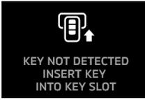
KEY NOT DETECTED<br>INSERT KEY INTO KEY SLOT | <ul style="list-style-type: none"> <li>The keyless operation key is not detected.</li> </ul>                                                          | <ul style="list-style-type: none"> <li>Insert the keyless operation key into the key slot.</li> <li>Refer to “If the keyless operation key is not operating properly” on page 6-21.</li> </ul> |
