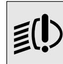
This warning lamp in the instrument cluster will illuminate when there is a fault in the LED headlamps.
