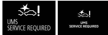
When the warning display appears, the Ultrasonic misacceleration Mitigation System does not operate normally because there are some malfunctions in the system or the sensor. Have the vehicle inspected at an authorised MITSUBISHI MOTORS dealer as soon as possible.
