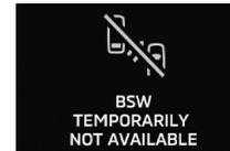
When the warning display appears, the sensor is temporarily not available for some reason such as the environmental condition or increase of the sensor temperature. When the warning display does not disappear after waiting for a while, contact an authorised MITSUBISHI MOTORS dealer.
