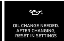
If the warning display appears, change the engine oil and reset the distance. For details on how to reset the distance, refer to "How to confirm and reset the distance until the next engine oil change" on page 6-22.
