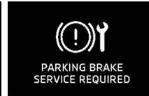
If there is a malfunction in the system, the Electric parking brake warning lamp will come on. In addition, the warning display appears on the information screen in the instrument cluster.
