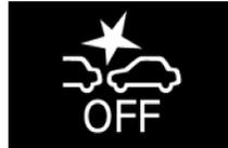
Even if you switch the FCM from ON to OFF, when the operation mode becomes ON, the FCM will be set ON.
