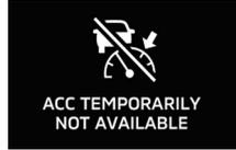
For example: The brake system is overheating due to continuous brake control on long downhill slope.
